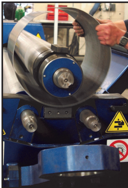
Above. Showing automated release of the work piece from the rolls.
