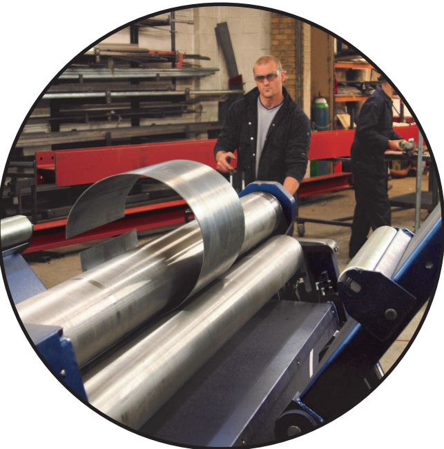
Below. Rolling in progress with the hydraulic loading supports contracting.
